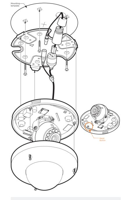
**Resetting the camera:** To reset the camera, use the tip of a paper clip or a pencil and press the reset button. Pressing the button for five (5) seconds will initiate a camera-wide reset of all the settings, including network settings.
