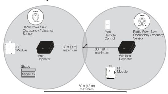
All devices must be located within 30 ft (9 m) of a repeater. The range can be extended with up to 4 Lutron wireless repeaters (Lx-REPPRO).
