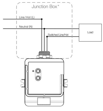
\* NOTE: Some applications (in USA) require the RF module to be installed inside an additional junction box. For information about how to perform this installation, please see Application Note #423 (P/N 048423) at www.lutron.com. Please consult all local and national electric codes for proper installation methods.
