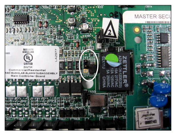
IMPORTANT: Remove the J600 shunt (circled) to change NAC D from 24V to 12V.
