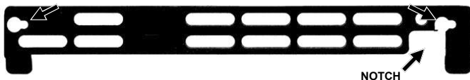
"KEYED" HOLES IN THE HW1764 POWER SUPPLY SHIELD (ARROWS). NOTE LOCATION OF "NOTCH".
