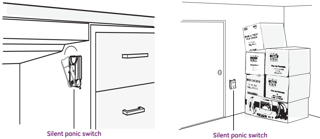
Figure 146. Panic switch installations
