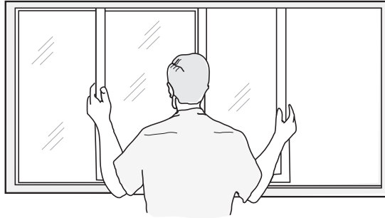
Figure 110. Window ventilation using two magnets
