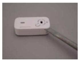
2. Insert the end of the screwdriver between the edge of the inner cover and the outer cover and carefully pry the inner cover off the sensor. Note: Insert the screwdriver into the side with the narrow ledge as shown in the picture below.
