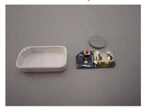
5. Install the new battery with the positive (+) side of the battery facing up, away from the circuit board.
