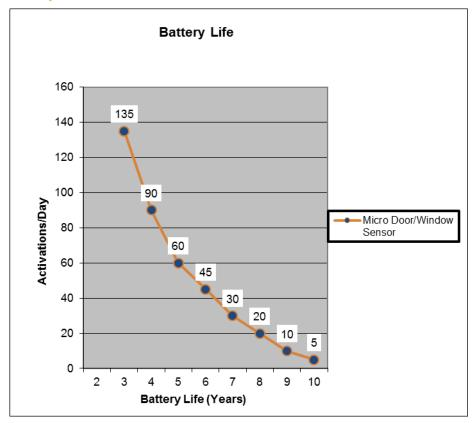
Battery life will vary, depending on the number of sensor activations. A sensor placed in a high-use area (for example, an entrance door with lots of traffic) will have a shorter battery life than a sensor place in an area used less often (for example, a rarely opened window).
