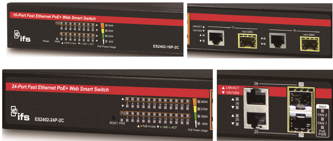
Figure 2-2 ES2402 SERIES LED panels
