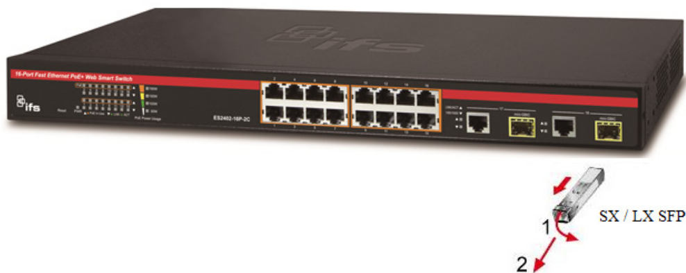
Figure 2-8 How to Pull Out the SFP Transceiver
