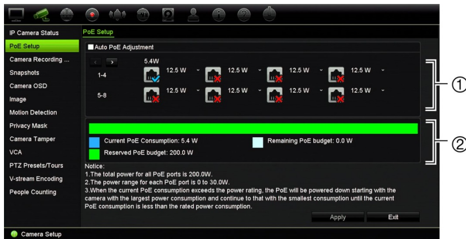
Figure 22: PoE power budget information on IP cameras
