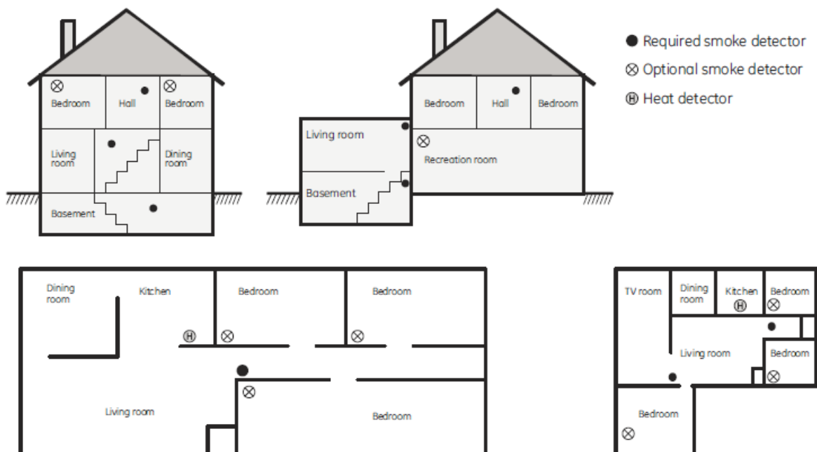
Figure 2. Smoke and Heat Detector Locations:
