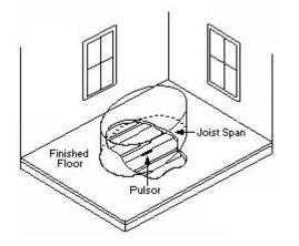
The Pulsor, stable and versatile, is also completely invisible. Mounted to the support joist *underneath* the floor, Pulsors can not be seen by intruders and do not have to be fitted to decor.
