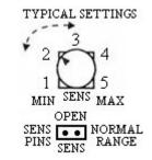
Walk-test the system. Walk-testing must be performed at each Pulsor location. Its purpose is to demonstrate that each Pulsor has enough sensitivity to protect its targeted area. Generally, an oval of protection (4' x 7") centered around the Pulsor is a typical stable configuration. Increase or decrease the sensitivity as necessary.
