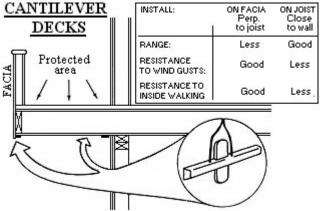
cantilever decks that are free form (no facia) must have Pulsors installed on the joist. These are more resistant to inside walking problem than boxed decks.
