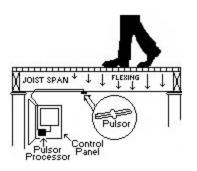
The Pulsor is a highly versatile motion sensing device that senses the physical flexing of whatever material it is epoxied to. Pulsors are environmentally sealed and utilize 22-gauge marine grade wire leads so they can be mounted both indoors and outdoors. They will not respond to shock, vibration, snow loads, building settling, airborne items or environmental conditions (including pets up to 60 pounds). They sense only the unique flexing of the floor caused by a person's movement.
