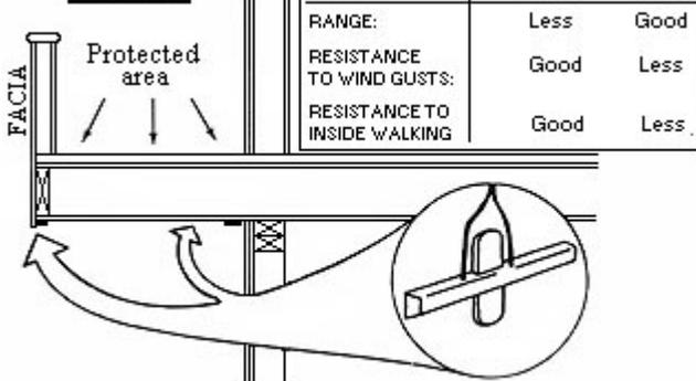
cantilever decks that are free form (no facia) must have Pulsors installed on the joist. These are more resistant to inside walking problem than boxed decks.
