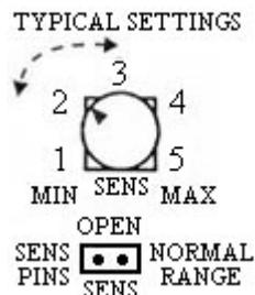
Walk-test the system. Walk-testing must be performed at each Pulsor location. Its purpose is to demonstrate that each Pulsor has enough sensitivity to protect its targeted area. Generally, an oval of protection (4' x 7") centered around the Pulsor is a typical stable configuration. Increase or decrease the sensitivity as necessary.
