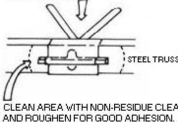
Use mixing stick to push squeezed epoxy back into joint.
