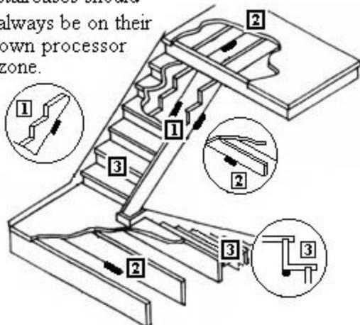
**Location 1: (Carriage):** Install 1/3 up (or down) on bottom of carriage. Side mount if to be drywalled.
