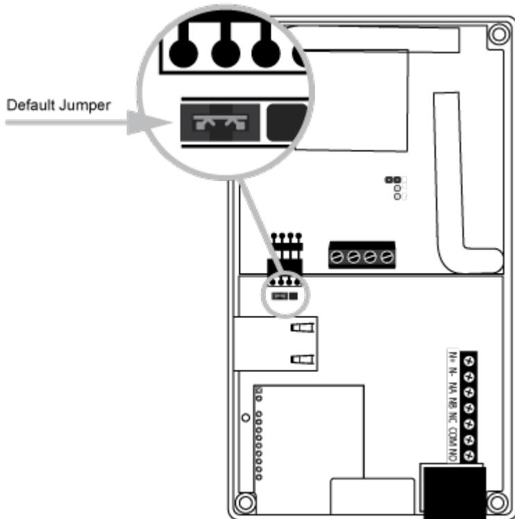
The jumper should be in the normal operating position on the two pins closest to the edge of the board.
