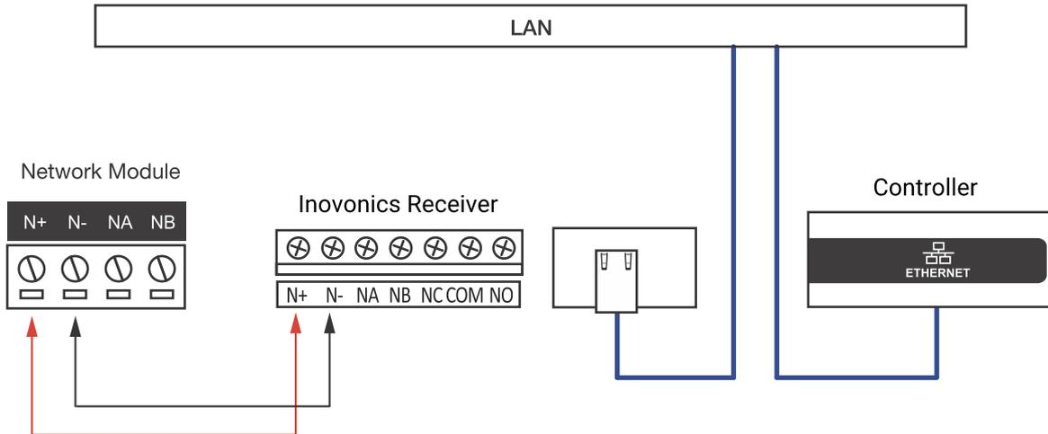
If the receiver module is inserted into an existing section of the RS-485 module network, both module and network power are supplied by the N+ and N- terminals.
