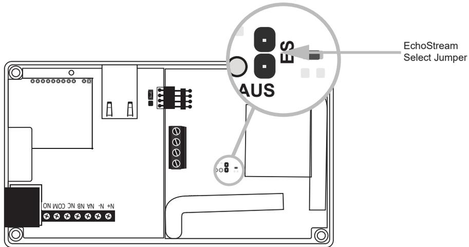
To enable EchoStream Select compatibility, place the jumper over the ES pins:
