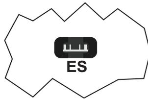
If there are no EchoStream Select products being used in your system, remove the jumper from the ES pins.
