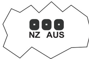
If using the device in **New Zealand**, place the jumper on the left two pins, marked NZ, to set the frequency range to 921-928 MHz:
