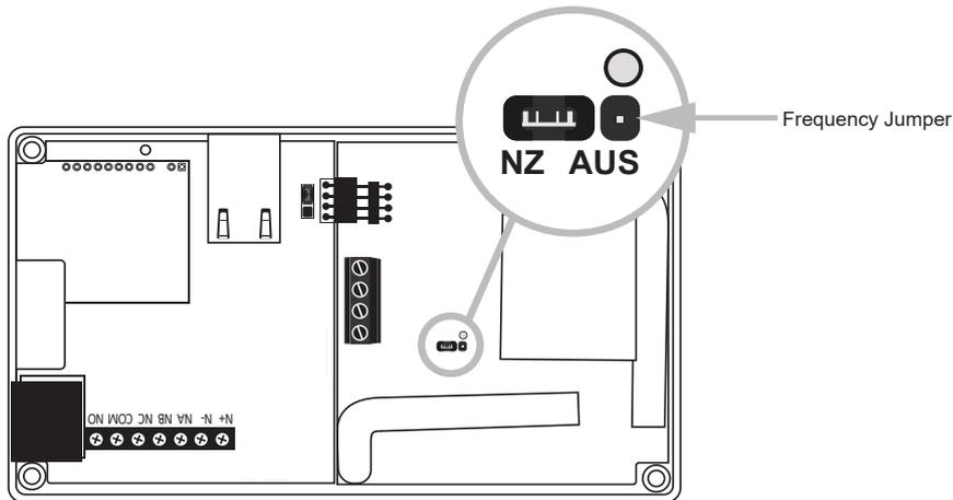
If using the device in **North America**, ensure that the frequency jumper is removed from the pins:
