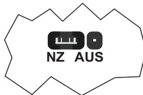
If using the device in **Australia**, place the jumper on the right two pins, marked AUS, to set the frequency range to 915-928 MHz:
