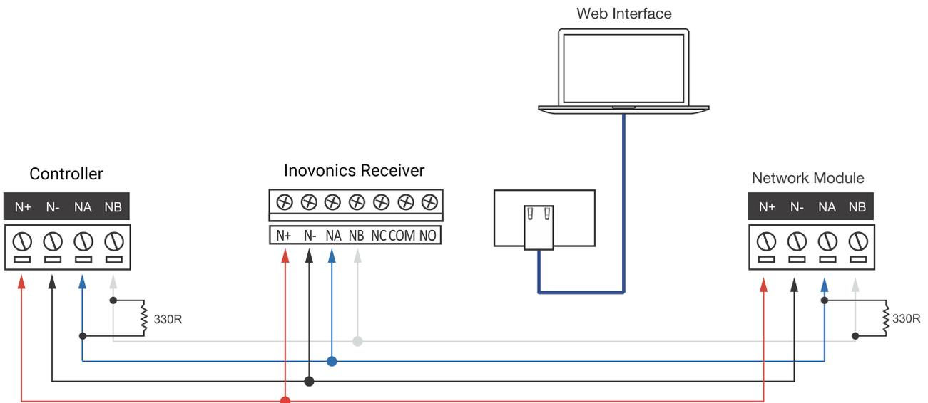
The 12V N+ and N- communication input must be supplied from only **one** point. Connections from more than one 12V supply may cause failure or damage to the unit or the device supplying network power.
