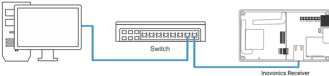
Temporary direct connections can be used for onsite programming by using a standard ethernet cable.
