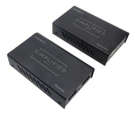
The EXUSB2.0 is a 40m (131ft.) US2.0 over category extender. The EXUSB2.0 is a plug and play device that requires no set up. The transmitter (TX) portion is powered via USB and has a USB Type-B port. Up to 10m more can be supported if the USB port is high powered that the TX is plugged into. The Receiver has two USB Type-A ports for the USB clients. The RX is powered with a 5V/1A power supply that is included in the kit.
