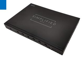
The MV2 is a compact 4 input to one output "frameless" switch. The MV2 has 4 HDMI Inputs and 1 HDMI Output. Switching can be accomplished by included IR remote or with IR commands from a third party control system. Switching is instantaneous. Output in quad mode is 4K. There are five output modes; single view, quad view, offset quad view, side by side, and a collaboration view as well.
