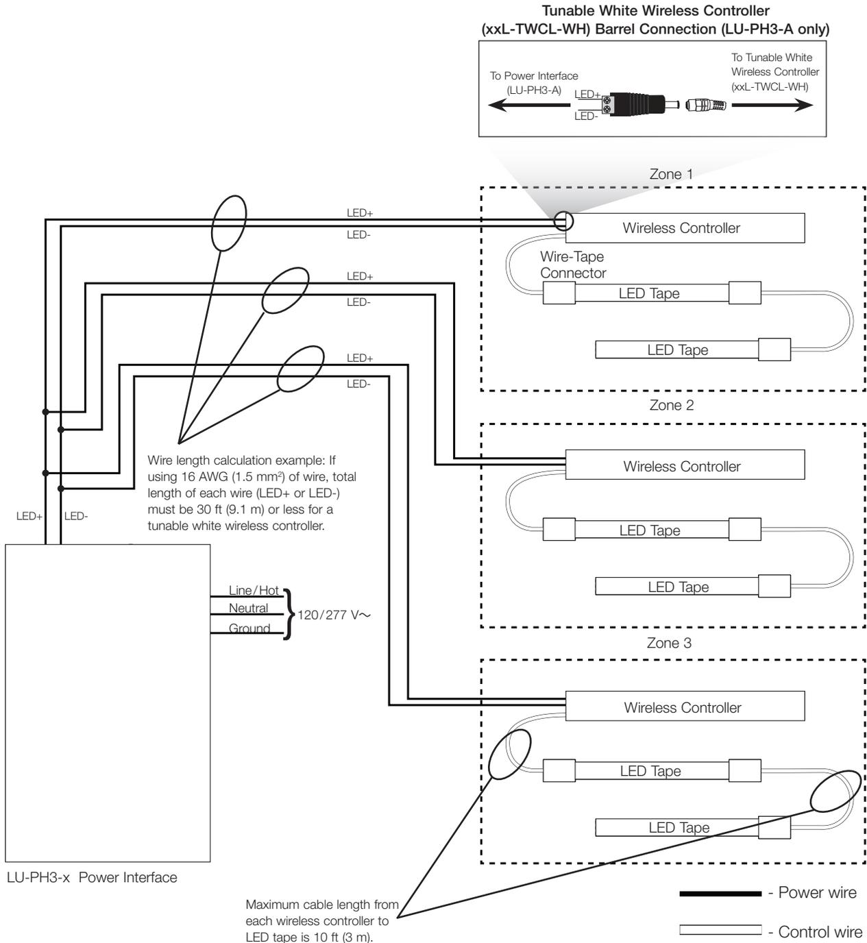
**Note: (LU-PH3-A only)** When wiring 3 zones (wireless controllers) to the power interface, two of the three wireless controller LED+ and LED- wires need to be spliced together in the power interface wiring compartment into a single wire run to the terminal block. LED+ and LED- terminals on the wireless controller accept one wire per terminal only.
