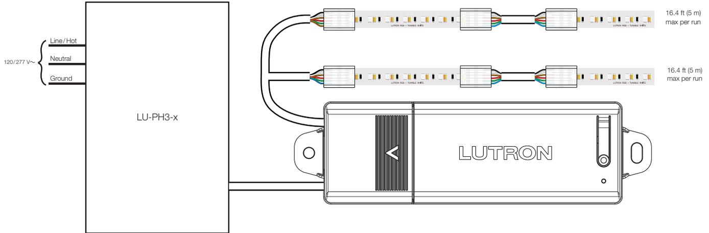
In this example, 32.8 ft (10 m) total of tape is wired to the multichannel controller. This is achieved here with two parallel runs, each 16.4 ft (5 m) long. Lengths greater than 16.4 ft (5 m) are not allowed. Since the RGB + Tunable White tape consumes about 2.9 W/ft and we have utilized 32.8 ft (10 m) of tape, the LU-PH3 is at its maximum rating of 96 W and another controller cannot be added to this interface. **Note:** All tape connected to the controller will be controllable as one fixture.
