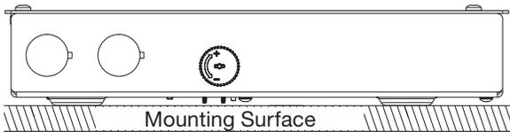
**Note:** The gray knob on the side of the enclosure is not used and does not need to be accessed after installation. This knob has no affect on the operation of the power interface.
