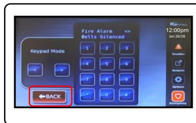
**Step 5:** Tap the 'BACK' button and Arm / Disarm the system to clear the alarm memory as needed.
